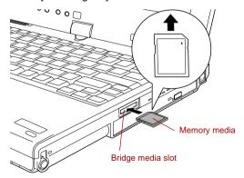
Figure 3-6 Inserting a memory media
